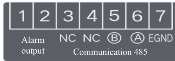
Fig.5 Blank type overall with communication type auxiliary wiring
